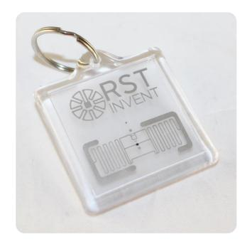
TwinTag-mini RFID tag is designed for use in solutions requiring stable registration of objects in three planes (3D format)
